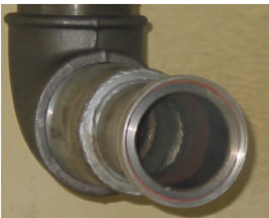
(c): The pipe terminal that was fastened to the high volume PM sampler
