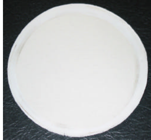
(a) Filter paper after 5 minutes collected from Engine # 1 (with soot-filter)
